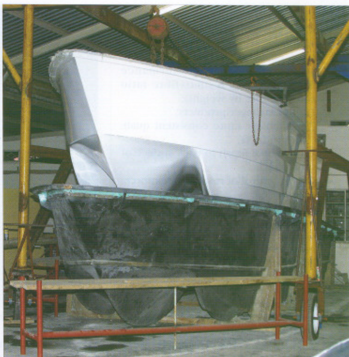
The finished product — the D7 hull — being removed from the mould.
