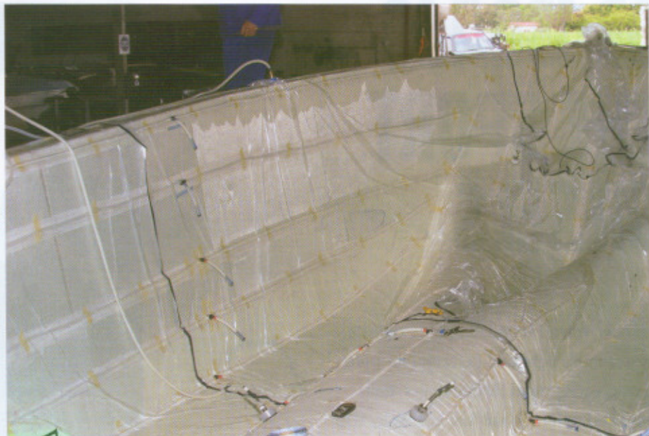
Resin being infused through the lay-up.
